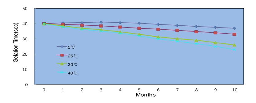
Gelation time is measured by Curelastometer method by using accurate stopwatch
