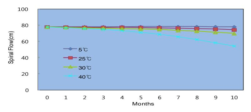
Spiral flow is measured based on the method of EMMI spiral flow mold(EMMI-1-66)
